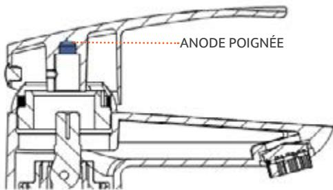
ANODE SITUÉE SUR LE FILETAGE DE L'EXCENTRIQUE, EN CONTACT AVEC TOUT LE CORPS D'UN BAIN OU D'UNE DOUCHE
