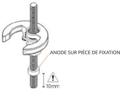
ANODE SITUÉE SUR LE FILETAGE DE FIXATION, EN CONTACT AVEC TOUT LE CORPS D'UN LAVABO OU D'UN EVIER
